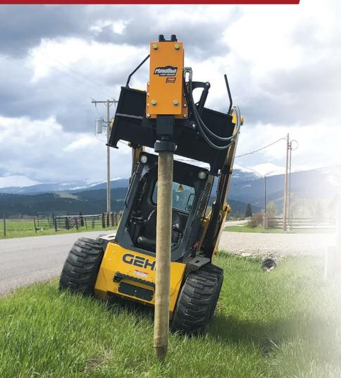
The Tilt attachment is an innovative mechanism that attaches to the Montana Post Driver between the driver and the mounting plate. A tilt plate driven by a hydraulic cylinder positions the Montana Post Driver to the desired angle. Fits models 750R, 1000E, and 1500E.
