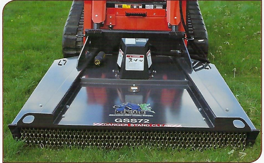
Available in 60" (standard flow), 72" (standard/high flow), and 78" (standard/high flow). Hydraulic couplers are included.
