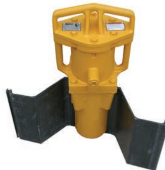
Driver shown with sheet pile inserted into chuck.
